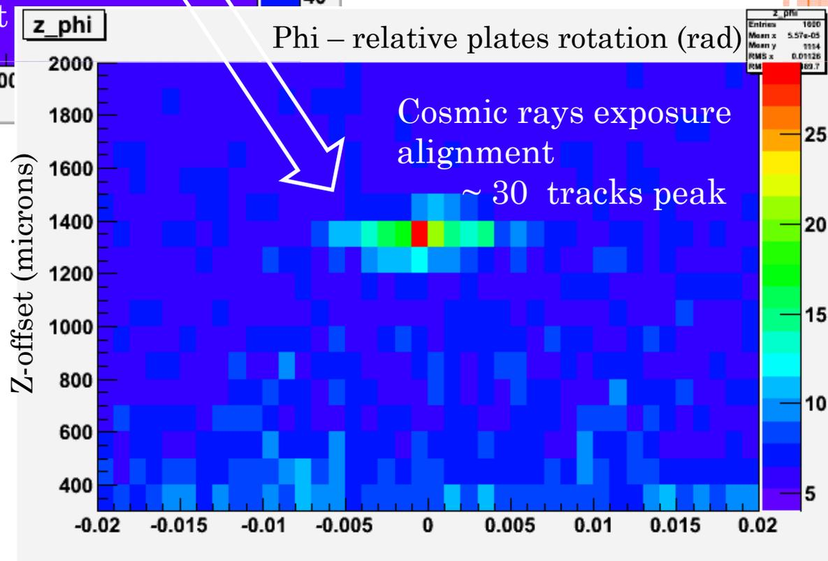
This procedure provides the position accuracy of about 0.5 -1.5 microns, depending on the zone size and the exposure time
