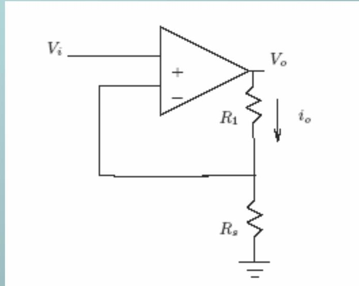
$$V_o = (R_1 + R_s)i_o = \frac{R_s}{(R_1 + R_s)} V_i$$
