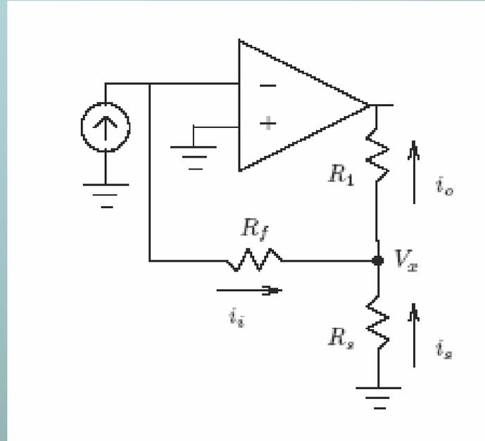
$$V_x = -i_i R_f = -i_s R_s ; i_o = i_i + i_s$$
