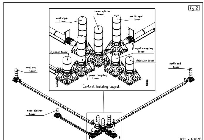
Figure 2 : Virgo layout with details of the central vacuum system
