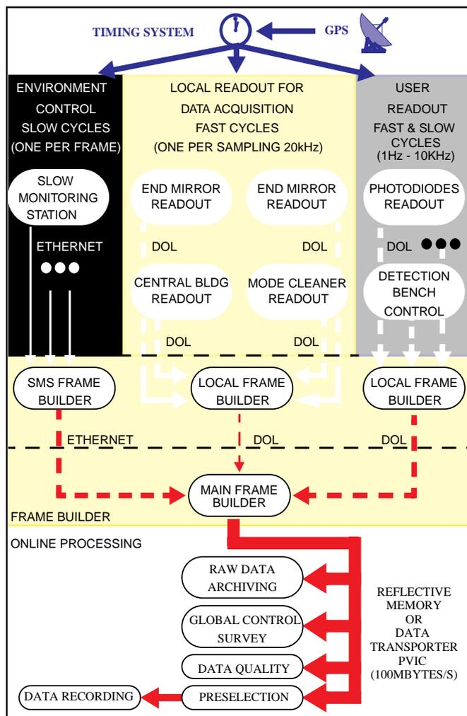
Figure 5: The Virgo data acquisition system
