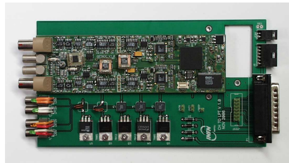
Figure 2. The Prototype of the Module in standalone configuration with the power distribution board. The hole in the power distribution base is to host the fan.
