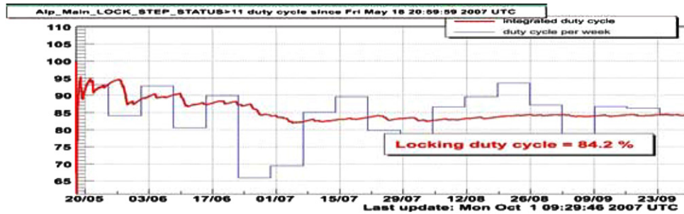
Figure 2. Duty cycle evolution during VSR1. The two lines represent the integrated duty cycle (continue-red line) and duty cycle per week (blue line). The Virgo interferometer was locked for the 84% and in science mode for 81% of its time.
