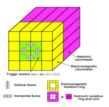
LVL1 Calo trigger based on the energy sum of cells belonging to a trigger tower reconstructed online  $1TT = 0.1 \times 0.1 \ \eta \times \phi$
