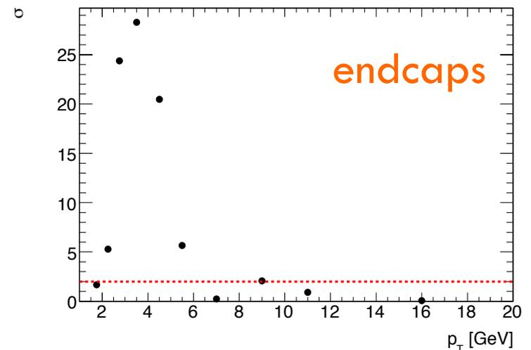
The two efficiency curve selecting muons with  $(q \cdot \eta) > 0$  and  $(q \cdot \eta) < 0$  are compatible for a  $p_T > 5 \text{ GeV}$ .
