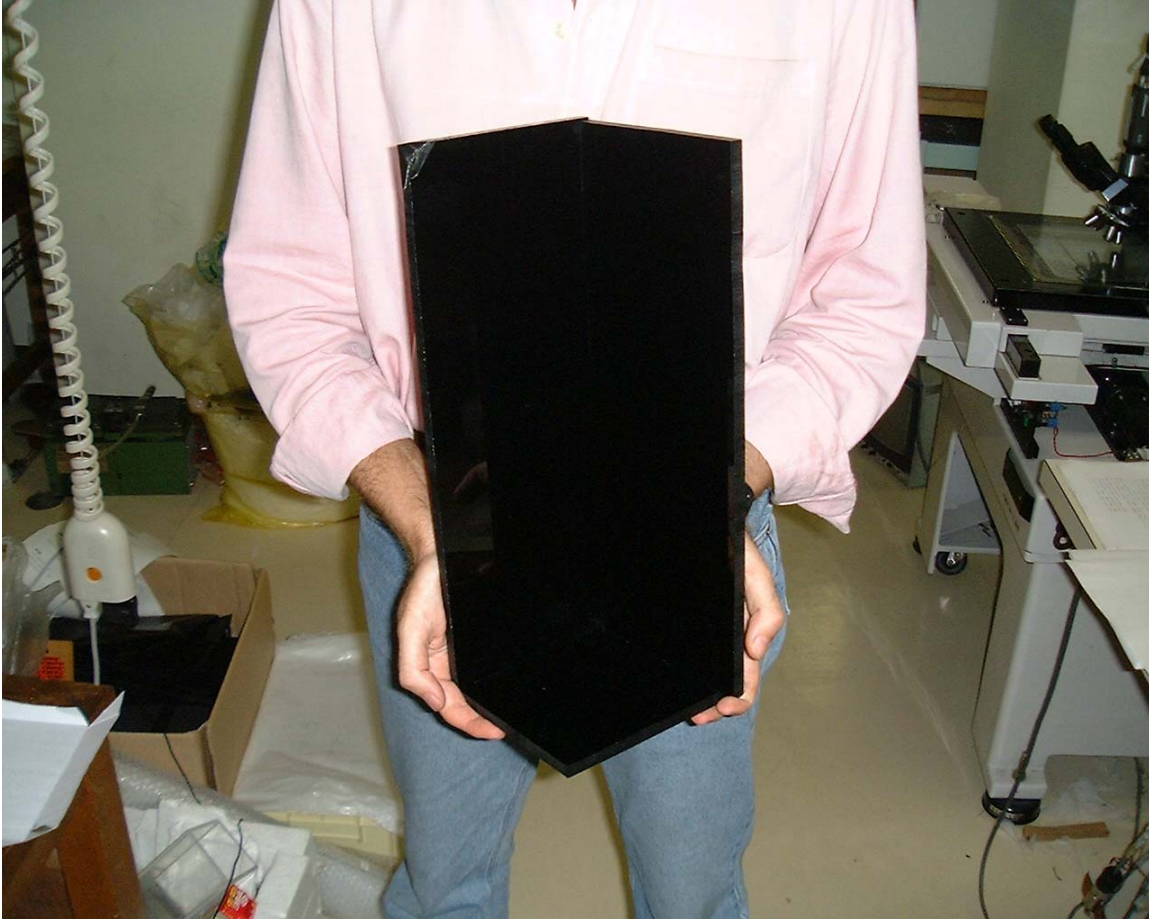
Figure 8: support for the piling-up of the chamber.
