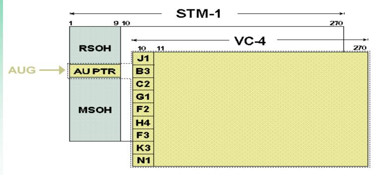
RSOH: Regenerator Section Overhead. MSOH: Multiplexer Section Overhead.
