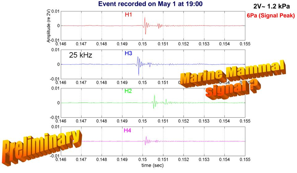
The exact position of the four hydrophones is known, this information will be used to locate the source position (direction)
