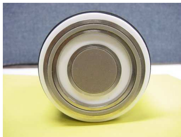
Figure 5: Concentric ring probe.
