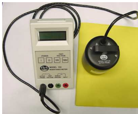
Figure 4: Surface resistivity measurement setup.
