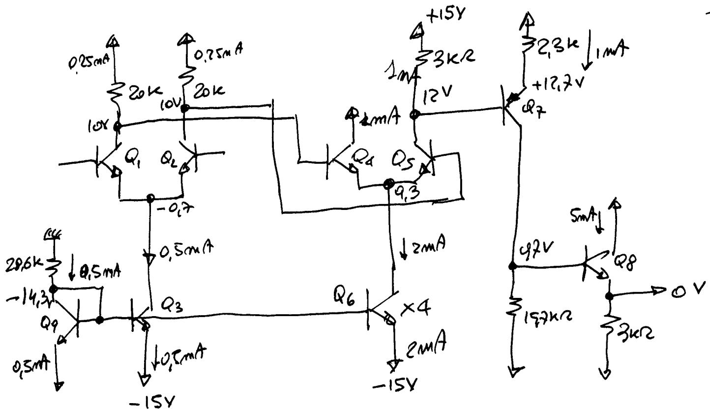
in  $Q_9$   $0.5\text{mA}$   $\Rightarrow$  anche  $Q_3 = 0.5\text{mA}$   $\Rightarrow Q_6 = 2\text{mA}$
