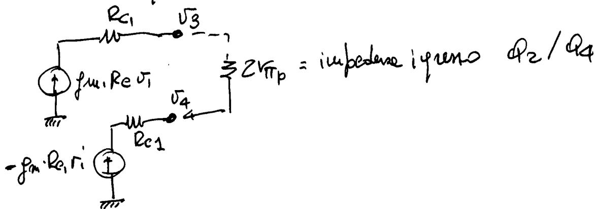
$$A_{\text{dm-se}} = f_m R_{C1} \frac{\frac{Z_{\text{mp}}}{2 R_{C1} + Z_{\text{mp}}}}{\frac{Z_{\text{mp}}}{2 R_{C1} + Z_{\text{mp}}} + 1} \cdot f_m R_C / 2$$
