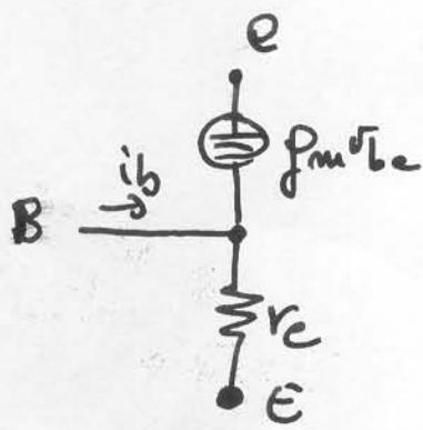
$$i_b = \frac{V_{be}}{r_c} - f_m V_{be} = \frac{V_{be}}{r_c} (1 - f_m r_c)$$
