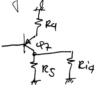
$$R_{i4} = I_{fe} \cdot (r_{es} + R_6) = 100 (55\Omega + 3k) = 303.5k$$
