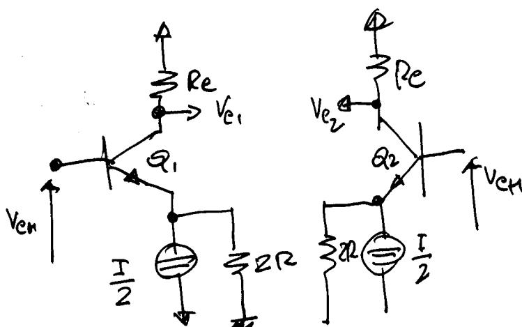
$$V_{ce1} = V_{cm} = \frac{R_c}{2R + r_c}$$
