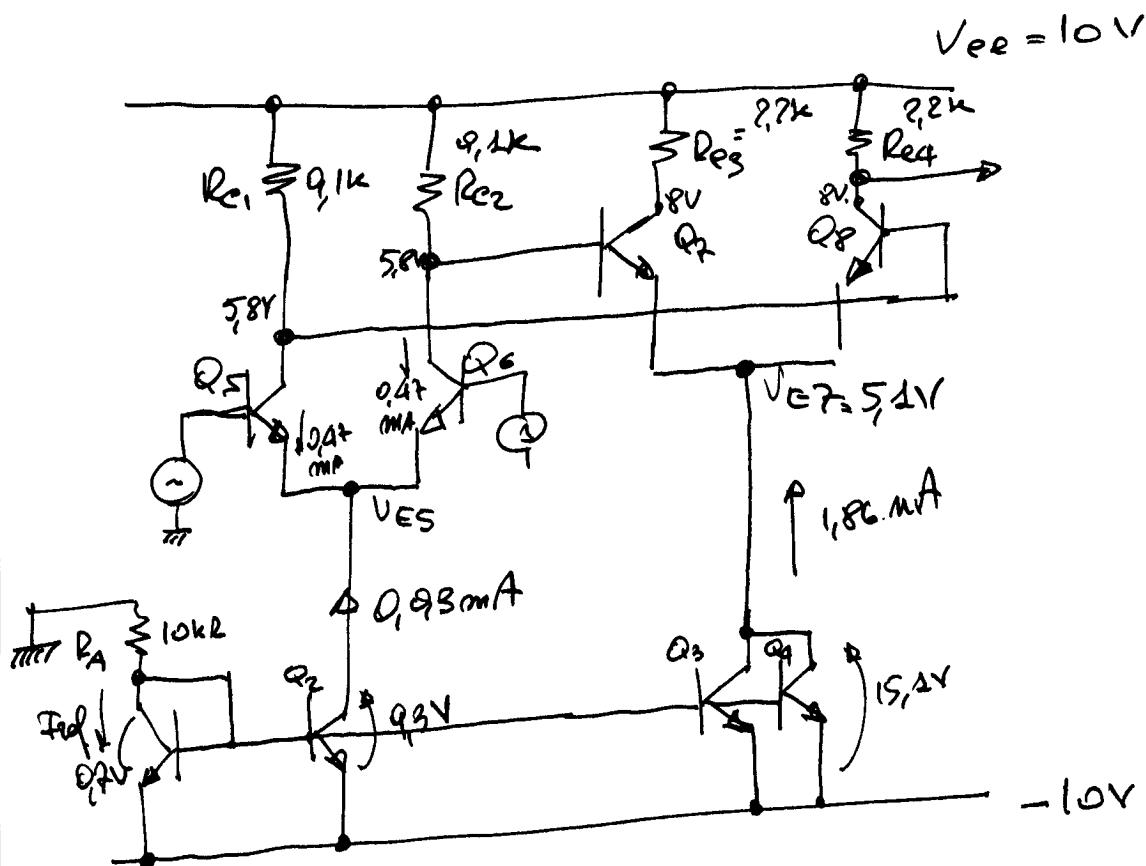
$$\textcircled{1} \quad I_{\text{ref}} = \frac{-Q_7 - (-10V)}{10k\Omega} = 0.93 \text{ mA} \quad (\text{prstazza})$$
