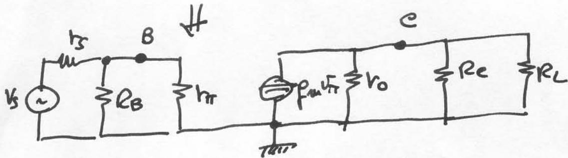
$$R_i = R_B \parallel r_\pi$$
