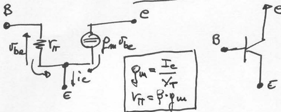
$$i_e = \frac{V_{be}}{r_\pi} + f_m V_{be} = \frac{V_{be}}{r_\pi} (1 + f_m r_\pi) = \frac{V_{be}}{r_\pi} (1 + \beta)$$
