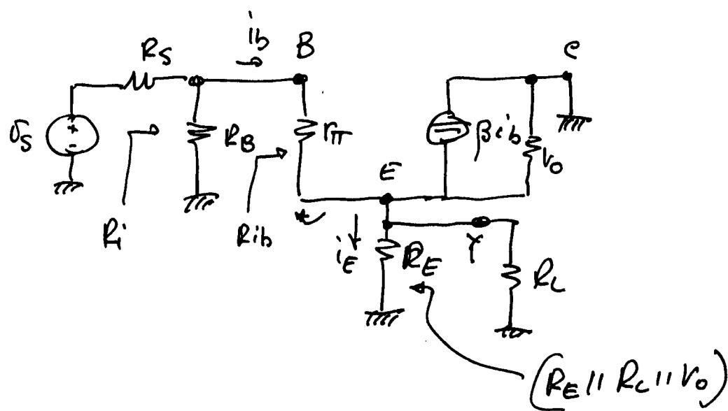
$$i_E = \beta i_b + i_b = i_b (\beta + 1)$$
