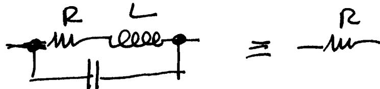
$$\text{Se } \omega L \ll R \text{ ed } \frac{1}{\omega C} \gg R$$
