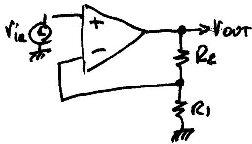
$$V_{out} = A(j\omega)(V_+ - V_-) = A(j\omega) \cdot \frac{R_1}{R_1 + R_2} \cdot (V_{in} - V_{out} \frac{R_1}{R_1 + R_2})$$
