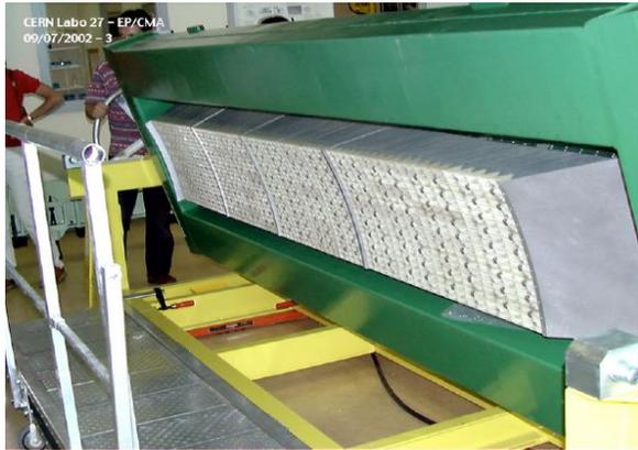
**A CMS Supermodule with 1700 tungstate crystals**
