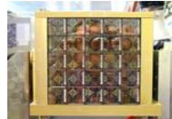
**A CMS endcap 'supercrystal' 25 crystals/VPTs**
