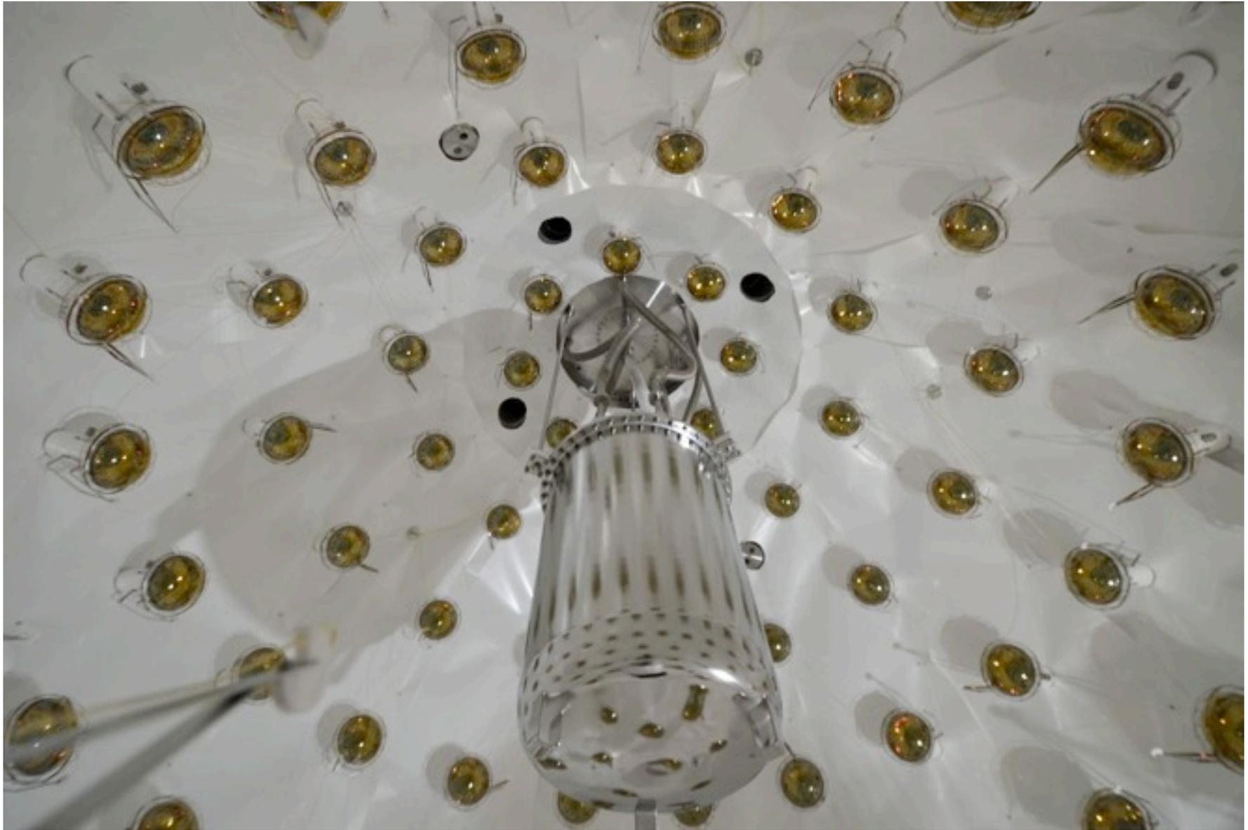
Cryostat containing the Time Projection Chamber hanging inside the neutron veto. The neutron veto sphere will be filled with boron-loaded liquid scintillator.
