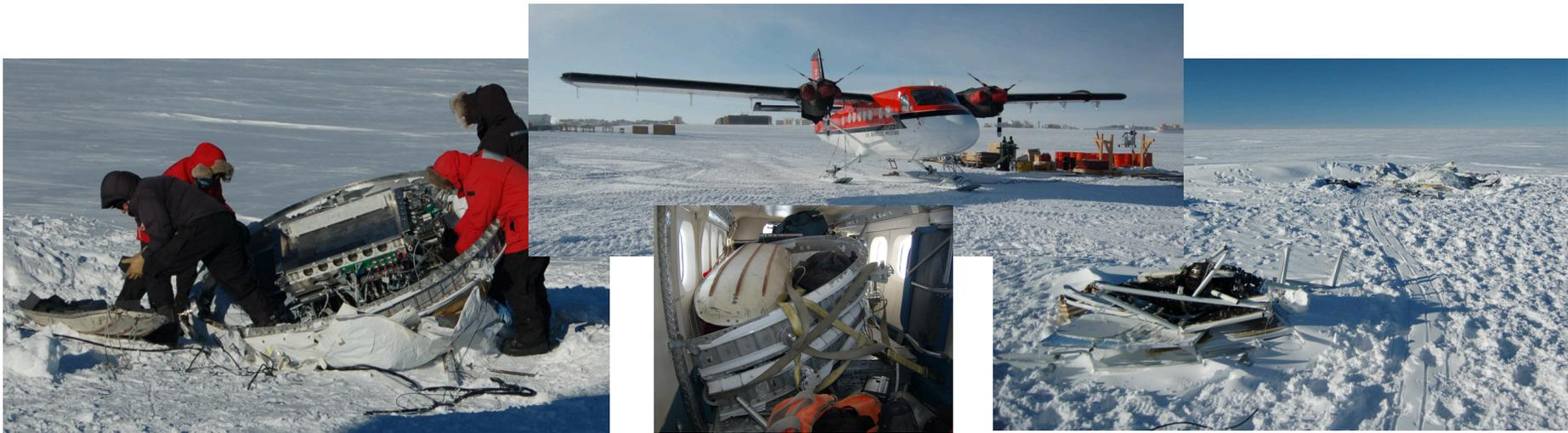
ATIC is designed to be disassembled in the field and recovered with Twin Otters. Two recovery flights are necessary to return all the ATIC components. Pictures show recovery flight of ATIC-4
