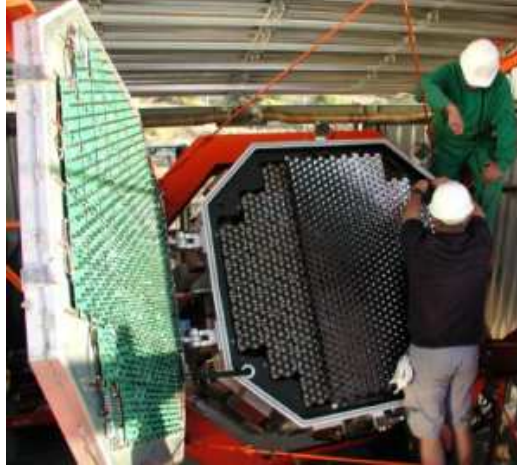
Abbildung 4.5: The H.E.S.S. Camera with the lid opened.
