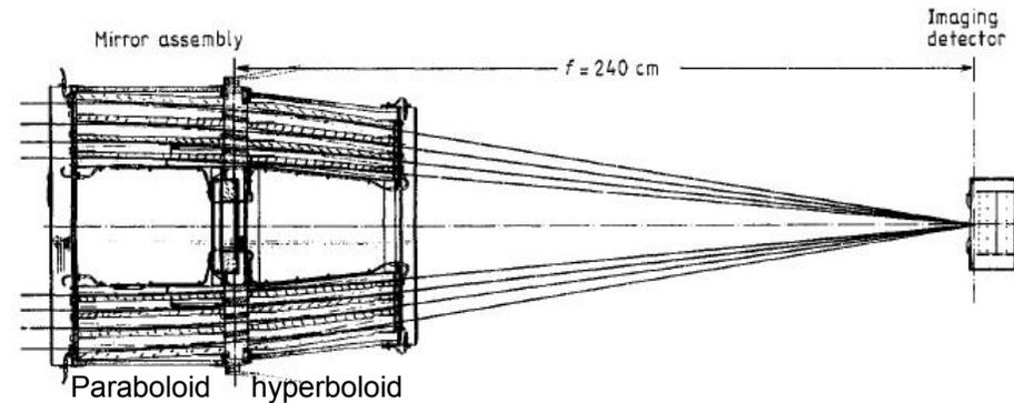
Figure 12. Schematic cross section of the Rosat telescope showing the four nested Wolter type I mirror systems. (from Aschenbach 1985 review)
