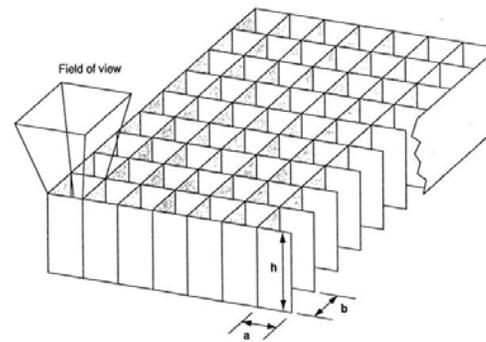
Slat collimator (**left**) with  $\text{FWHM} = \tan^{-1}(a/h) \times \tan^{-1}(b/h)$  vs. modulation collim. (**right**) (from Ramsey et al review)
