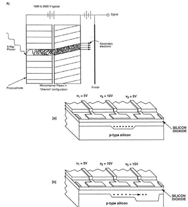
Fig. 3.14. Diagram illustrating how charge is transferred in a three-phase charge coupled device (CCD). (a) Electrons lie in the potential well formed by high voltage on  $v_2$ . (b) Increased voltage on  $v_3$  causes charge to be transferred to the lower potential region.
