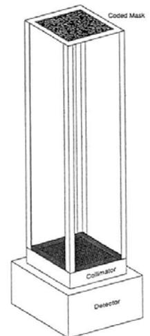
Schematic coded mask teles.
