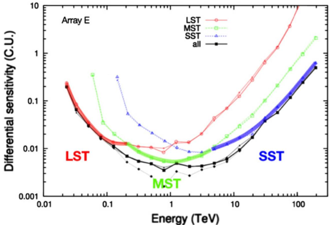
CTA performance below  $\sim 100$  GeV is given by LSTs and we aim to go down to 20 GeV
