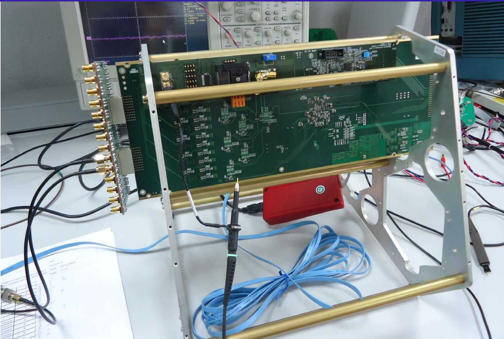
**Dragon board V4 (version for 1<sup>st</sup> telescope, Kyoto+Pisa) has been tested together with trigger and backplane
