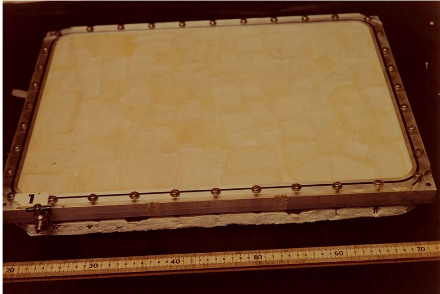
A single large area detector tray made from NaI (TI) Crystal pieces
