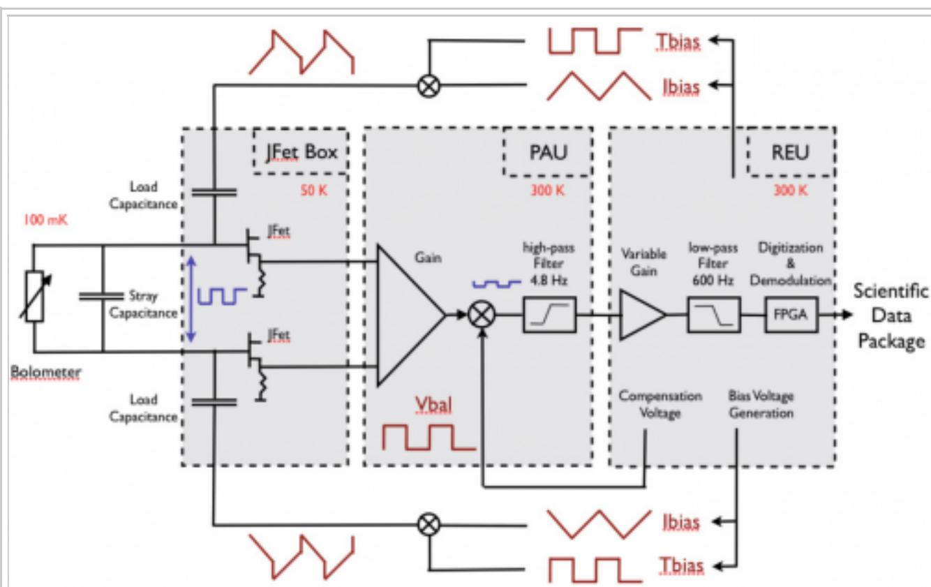
Principles of readout electronics. The three modules of the chain are shown: JFET box; Pre-Amplifier Unit (PAU); and Readout Electronic Unit (REU)
