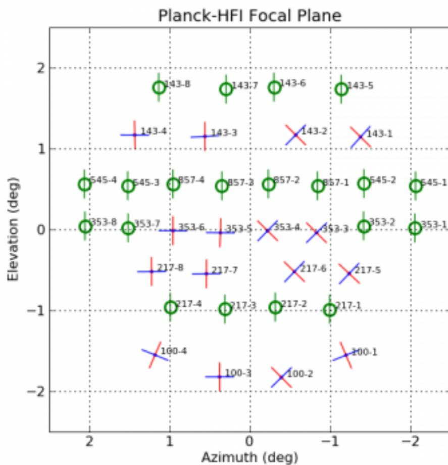
Focal plane layout as seen from outside the celestial sphere. PSB orientations are indicated, with a red rod for the "a" elements and a blue rod for the "b" elements. The scan direction is from left to right.
