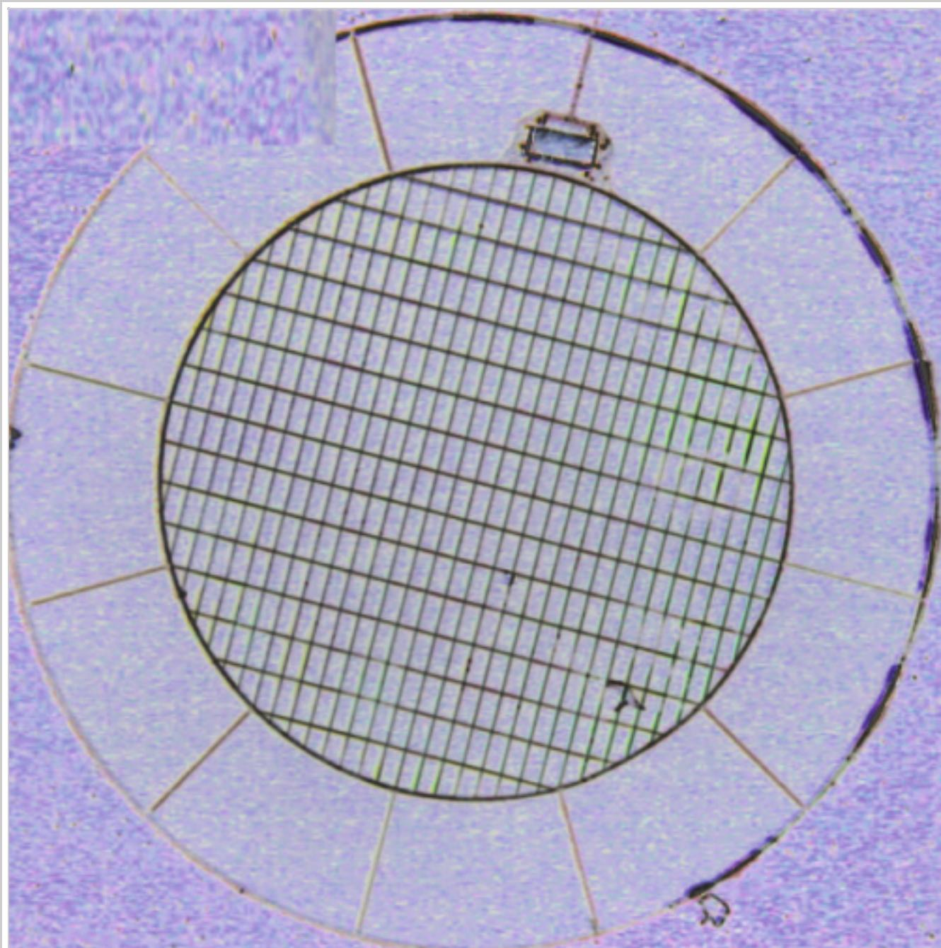
Picture of a polarization-sensitive bolometer. This is a 217 GHz module. The temperature sensor is located at one edge of the absorbing grid.
