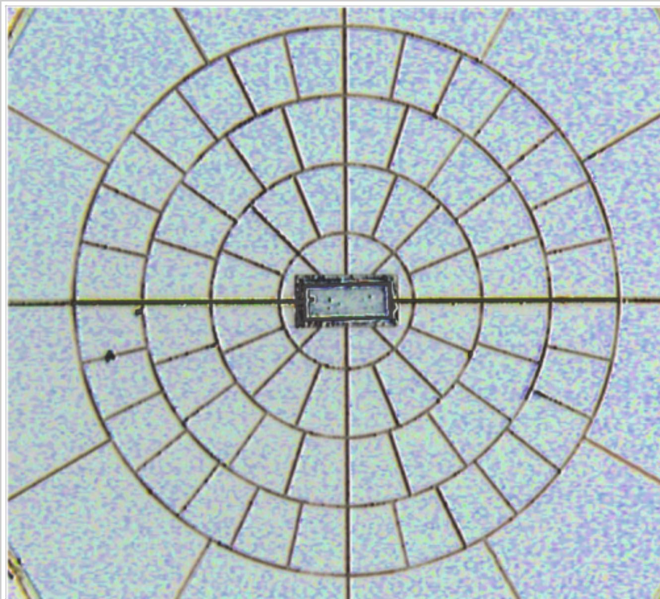
Picture of a spider-web bolometer. This is a 143 GHz module. The temperature sensor is at the centre of the absorbing grid.
