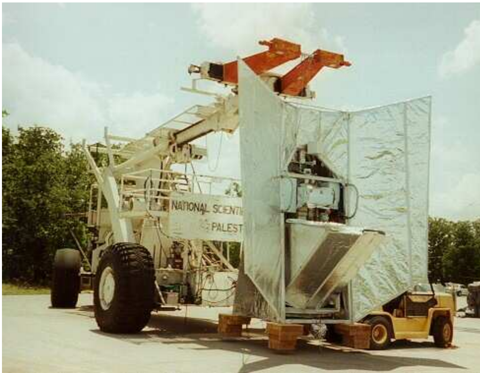
Fig. 2. The BOOMERanG payload hanging from the launch vehicle on Aug.30, 1997. The earth shield and the two sun shields dominate the scene.
