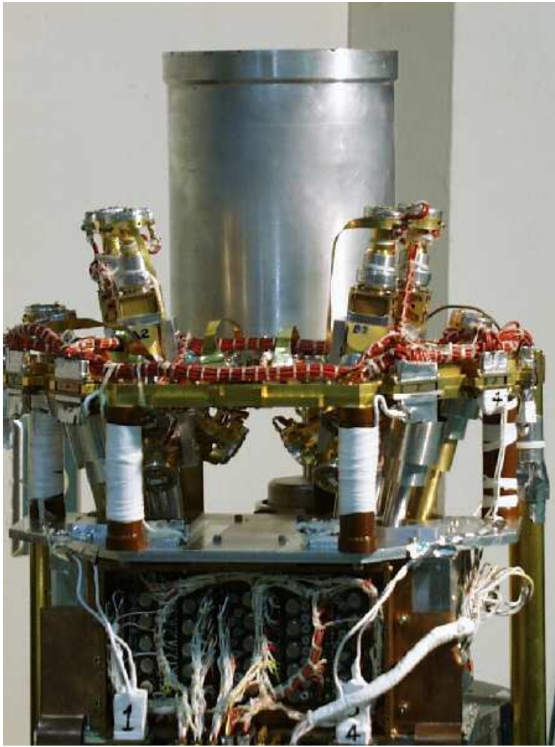
Fig. 3. The cryogenic insert for the BOOMERanG 1998 receiver. The gold plated flange is supported by vespel columns and is cooled to 0.28K by the ^3\text{He} fridge visible in the background. Above the flange the multiband photometers and the related wiring are visible. Below the flange is visible the cryogenic preamplifier box (lid open). The insert shown in the picture is 60 cm high and is bolted on the 2K flange of the main long duration dewar.
