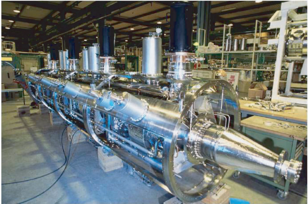
Figure 14. Four-cavity module during assembly.
