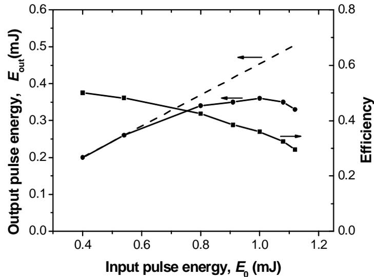
Fig. 7. Measured pulse energy at the fiber output and measured efficiency of optical propagation through the hollow fiber as a function of the input pulse energy. Solid circles and line: pulse energy at the fiber output versus the input pulse energy. Squares and solid line: optical propagation efficiency versus the input pulse energy. Dashed line: theoretical pulse energy at the fiber output in the case of propagation of the pure fundamental fiber mode.
