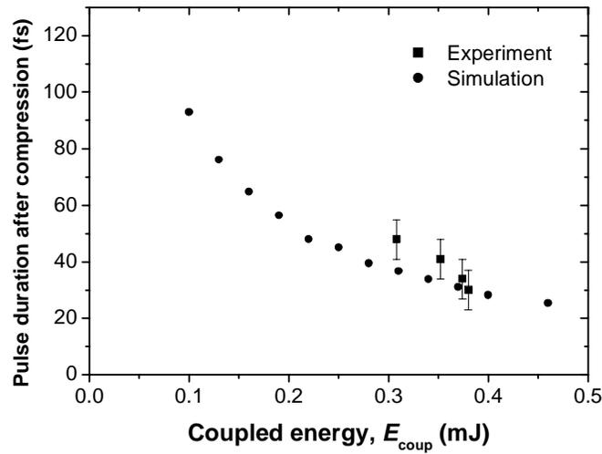
Fig. 4. Pulse duration versus the pulse energy coupled into the fiber.
