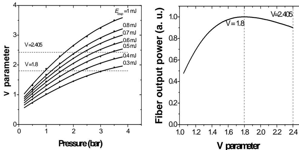
Fig. 8. (a) Normalized frequency versus filling-gas pressure at the differently initial pulse energy. (b) Fiber output power in the fundamental mode
