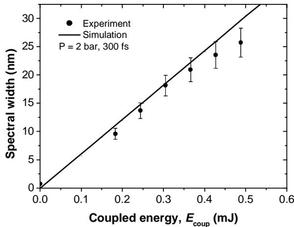
Fig. 3. Spectral width of the fiber output pulses as a function of the coupled energy.
