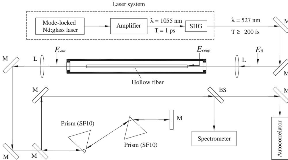
Fig. 1. Scheme of the experimental setup. BS: beam splitter; L: lens; M: mirror.
