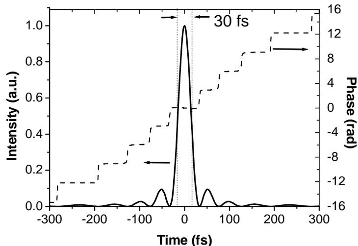
Fig. 6. Retrieved temporal shape of the pulse intensity profile (solid) and phase (dashed).
