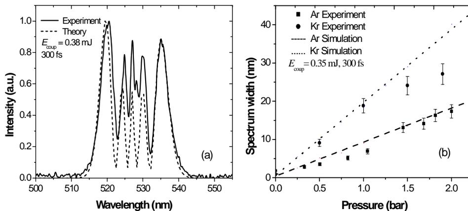
Fig. 2. (a) Measured (solid) and corresponding simulated (dashed) pulse optical spectrum in the best experimental conditions. (b) Spectral width.
