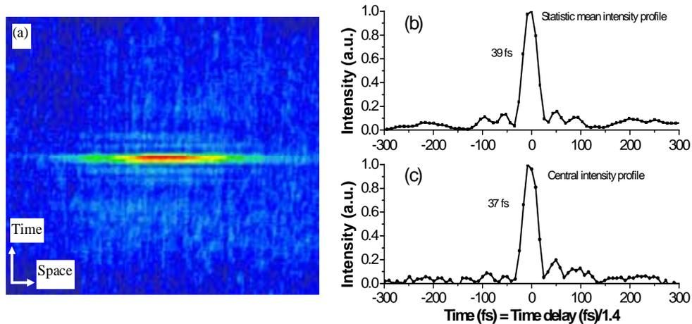
Fig. 5. (a) 2D autocorrelation pattern of the compressed pulses. (b) Spatially integrated autocorrelation traces of the compressed pulse. (c) Autocorrelation trace of the compressed pulse as read at the spatial centre of the wavefront.
