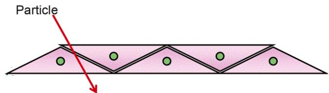
**Fig. 16.** The scintillators of the MINERvA inner detector.
