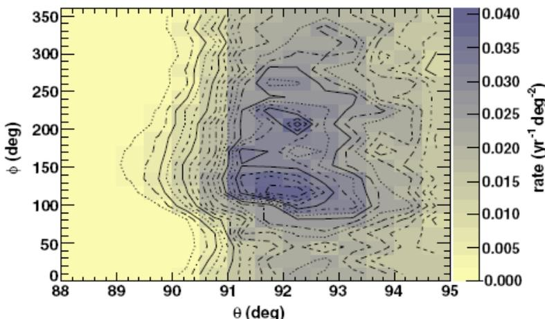
**Fig. 5.** Event rate as a function of azimuth and zenith for the active Auger volume, in the case of Earth-skimming  $\nu_\tau$  showers ( $85^\circ < \theta < 95^\circ$ ) assuming  $E^{\text{thr}} = \mathcal{O}(\text{EeV})$  for the  $\tau$  [32].
