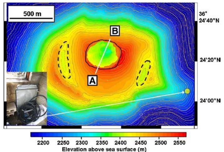
**Fig. 8.** Map of Mt. Asama with the location of the cosmic ray muon detector indicated by an arrow. The line A-B shows the vertical cross-sectional plane as seen by the detector [7].
