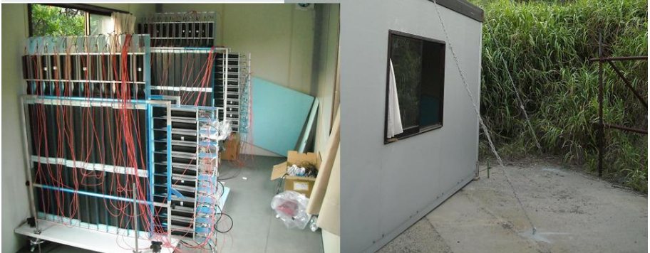
Fig. 18. The experimental set-up for the muon radiography of the Satsuma Iwo-jima volcano.
