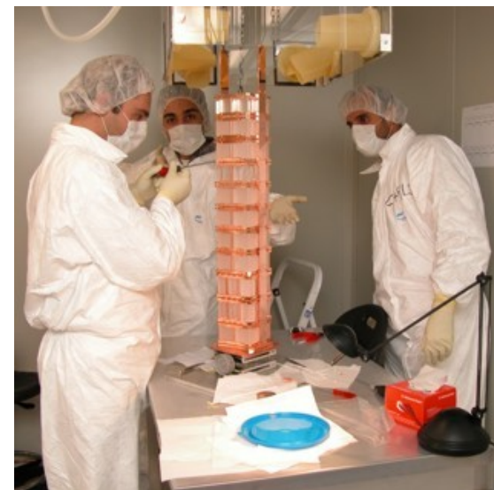
The Cuoricino \text{TeO}_2 array 41 kg \text{TeO}_2 crystals
