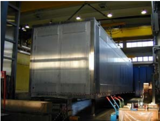
The ICARUS T600 detector 600 t liquid Ar TPC
