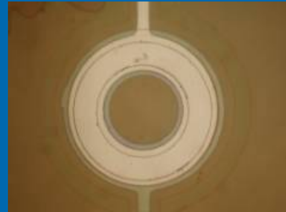
Photograph annular junction R=45\mu\text{m} . R_{\text{int}}=30\mu\text{m} , \lambda_j \sim 45\mu\text{m} IC-C.N.R.
