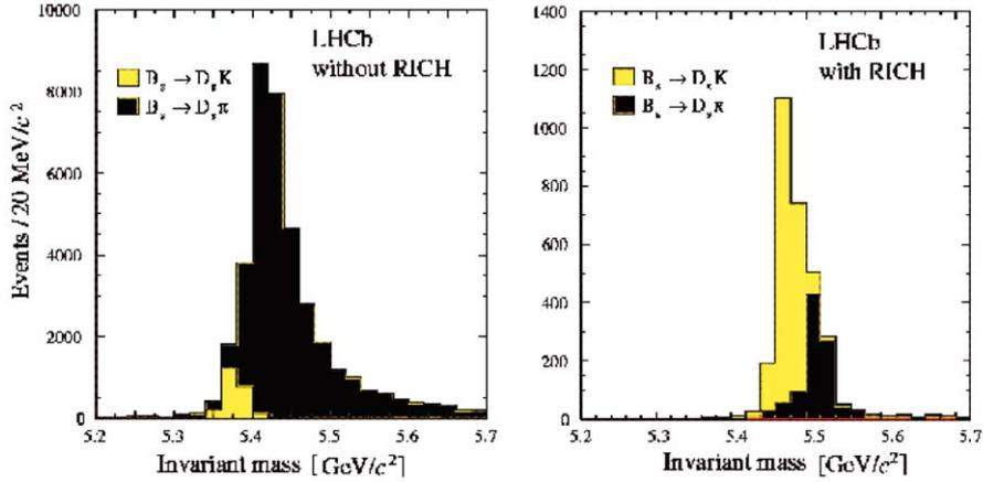
Fig. 3. The reconstructed  $B_s \rightarrow D_s K$  mass spectrum (gray histogram) on top of the  $B_s \rightarrow D_s \pi$  background (black histogram), obtained from a simulation of the LHCb experiment without (left panel) and with (right panel) the information of the RICH detectors.
