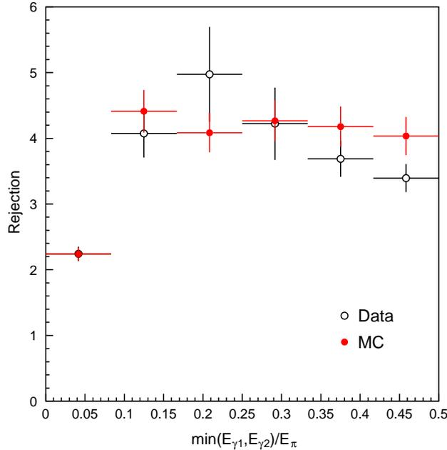
Fig. 7. Rejection against  $\pi^0$  with  $p_T \sim 50$  GeV, for a 90% efficiency for single photons, as a function of the energy fraction carried by the less energetic photon. The open symbols show results from test-beam data collected with final modules of the ATLAS liquid-argon electromagnetic calorimeter and a special photon beam, whereas the dots indicate the prediction of the Geant3 simulation.
