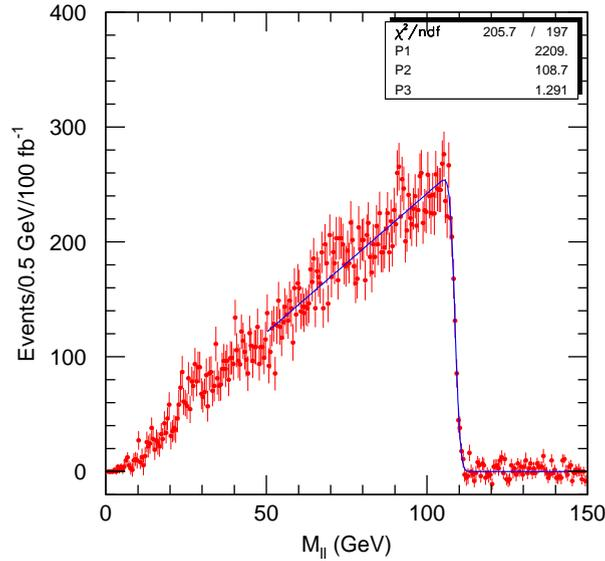
Fig. 10. Invariant mass distribution of  $e^+e^-$  and  $\mu^+\mu^-$  pairs at “Point 5” of mSUGRA (see text), as obtained from an ATLAS simulation for an integrated luminosity of  $100\text{ fb}^{-1}$ .
