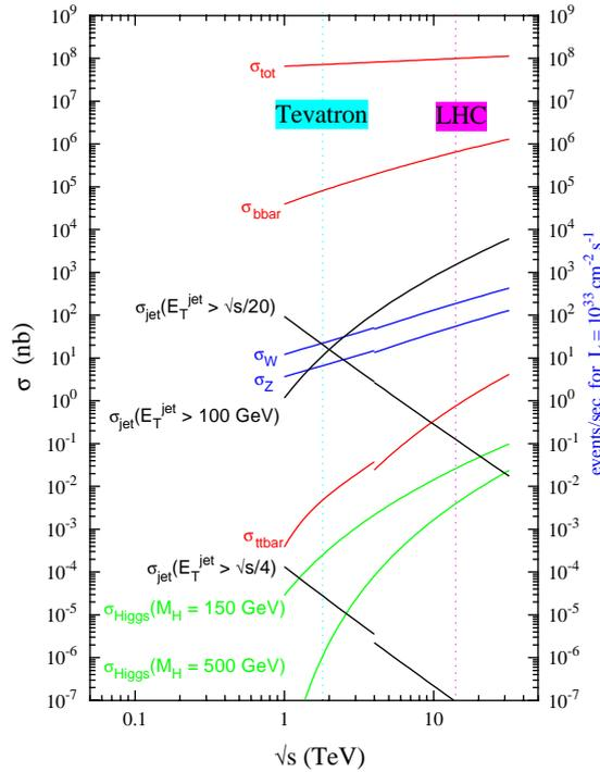
Fig. 1. Production cross-sections for various processes at hadron colliders ( $pp$  and  $p\bar{p}$ ), as a function of the machine centre-of-mass energy. The discontinuities in some of the curves are due to the transition from  $p\bar{p}$  to  $pp$  collisions.
