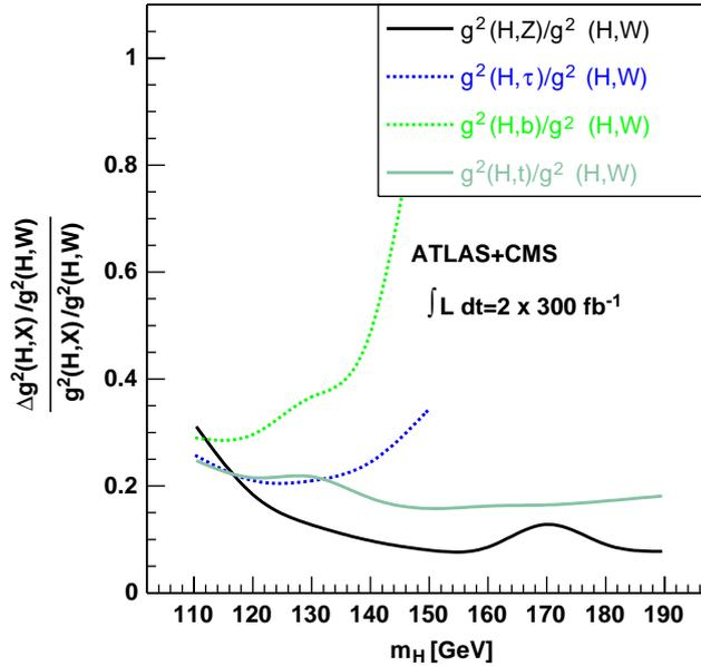
Fig. 8. The expected experimental precision on the measurements of ratios of Higgs couplings to fermions and bosons at the LHC, as a function of mass and for an integrated luminosity of  $300 \text{ fb}^{-1}$  per experiment. Systematic uncertainties are included.
