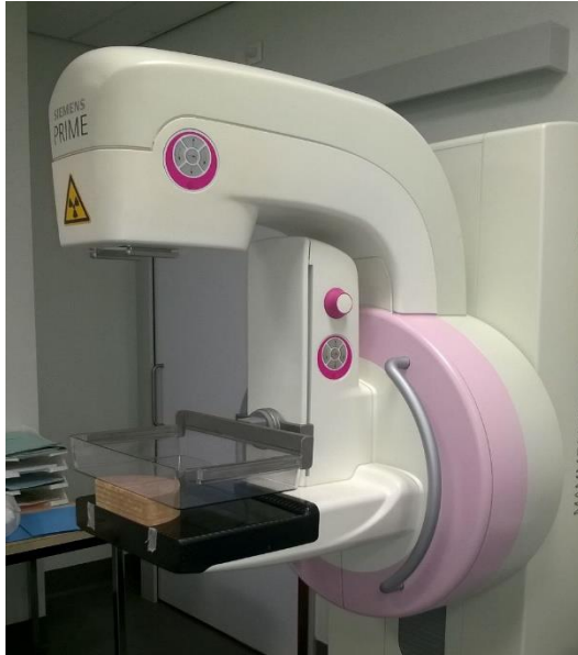
Siemens Mammomat Prime Anode/filter: W/Rh Scan angle: 50° Source-detector distance: 65 cm
