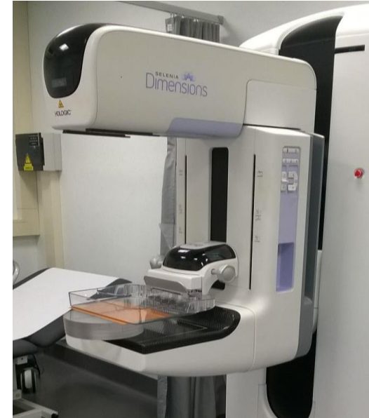
Hologic Selenia Dimensions Anode/filter: W/Al Scan angle: 15° Source-detector distance: 70 cm
