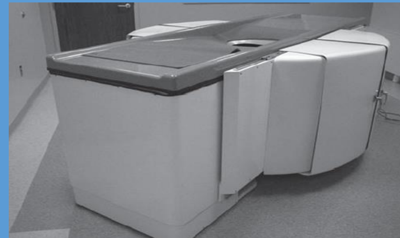
University of Rochester (Prof. R. Ning) Koning Corp. commercial scanner (FDA/EU approved for diagnostic imaging in combination with mammography, non contrast) 49 kVp
