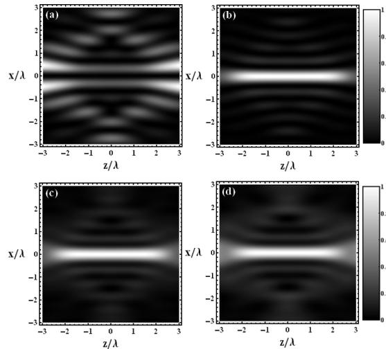
Fig. 3. Density plots of intensity distribution for (a) radial, (b) longitudinal components. (c) and (d) show the total intensity distribution for the HyGG-II<sub>-1,1</sub> and the BG<sub>1</sub> beams, respectively.
