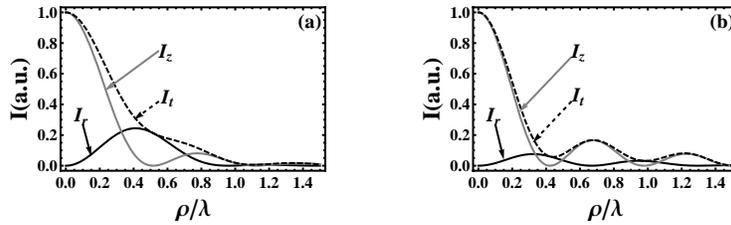
Fig. 2. Intensity profile of the longitudinal and radial field components at the focal point of a high numerical aperture lens (a) and a system of high numerical aperture lens and binary phase mask (b). The black, gray and dashed lines are radial, longitudinal and total intensity, respectively.
