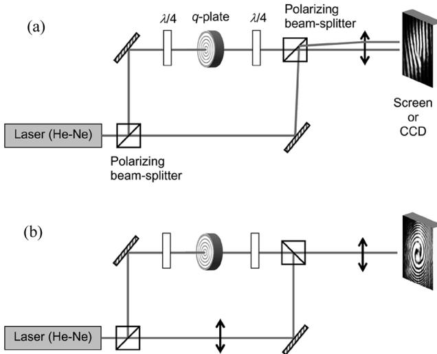
**FIGURE 4** Sketch of the Mach-Zehnder setup employed for proving the generation of helical modes and the corresponding conversion of angular momentum. (a) First layout, with slightly misaligned arms of the interferometer. (b) Second layout, with the reference beam having a different wavefront curvature from the signal beam, as obtained by inserting a lens in its arm.
