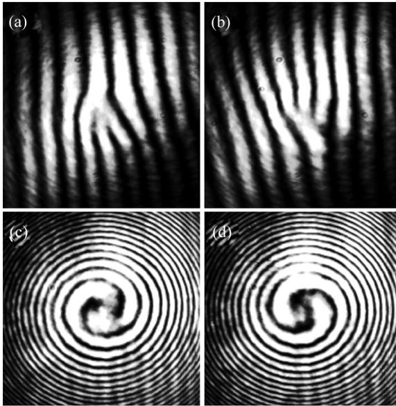
**FIGURE 5** Recorded interference patterns generated by the  $q$ -plate with  $q = 1$ . (a–b) panels refer to the first layout (plane-wave reference geometry, see Fig. 4a), (c–d) panels to the second one (spherical-wave reference, see Fig. 4b). Panels on the left, (a) and (c), are for a left-circular input polarization and those on the right, (b) and (d), for a right-circular one.
