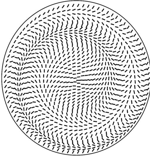
**FIGURE 6** Easy axis geometry of a hypothetical liquid crystal planar cell behaving as a (polarization-dependent) PBOE lens. Dashes indicate local director for a selection of radii. A perfect PBOE-lens will actually have a continuous variation of the optical axis.
