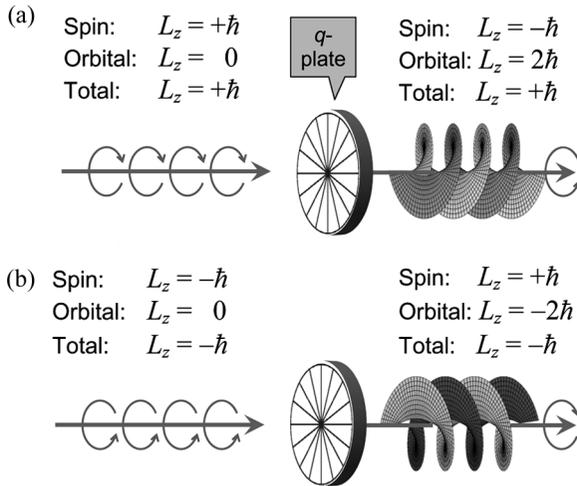
**FIGURE 3** Pictorial description of the spin-to-orbital angular momentum conversion occurring in a  $q$ -plate with  $q = 1$ , for a single photon. (a) Left-circular input polarization. (b) Right-circular input polarization.
