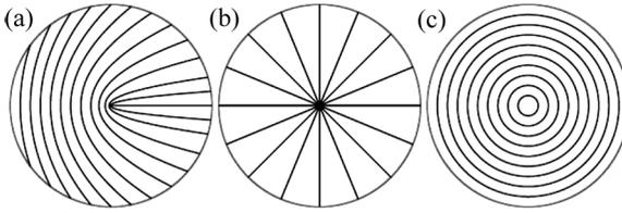
**FIGURE 2** Examples of  $q$ -plates. The tangent to the lines shown indicate the local direction of the optical axis (molecular director)  $\mathbf{n}$ . (a)  $q = 1/2$  and  $\alpha_0 = 0$  (a nonzero  $\alpha_0$  is here just equivalent to an overall rigid rotation), which generates helical modes with  $m = \pm 1$ ; (b)  $q = 1$  with  $\alpha_0 = 0$  and (c) with  $\alpha_0 = \pi/2$ , which can be both used to generate modes with  $m = \pm 2$ .
