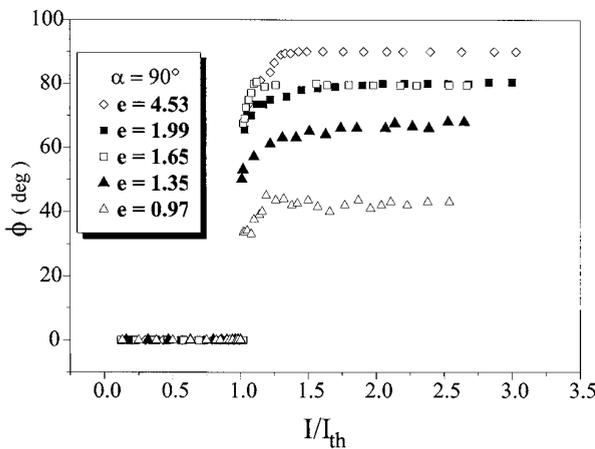
**Figure 7.** Steady-state value of the director average azimuthal angle  $\phi$  as a function of the reduced laser intensity  $I/I_{th}$  for different values of  $e$  of the unpolarized beam spot at the sample. The spot ellipse major axis was oriented at  $\alpha = 90^\circ$ . Below threshold ( $I/I_{th} < 1$ ), the angle  $\phi$  has no physical meaning.
