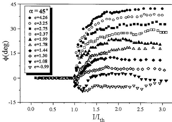
**Figure 9.** Steady-state value of the director average azimuthal angle  $\phi$  as a function of the reduced laser intensity  $I/I_{th}$  for different values of  $e$  of the unpolarized beam spot at the sample. The laser beam was linearly polarized in the horizontal plane  $\phi = 0$  and the spot major axis was oriented at  $\alpha = 45^\circ$  with respect to the same plane.
