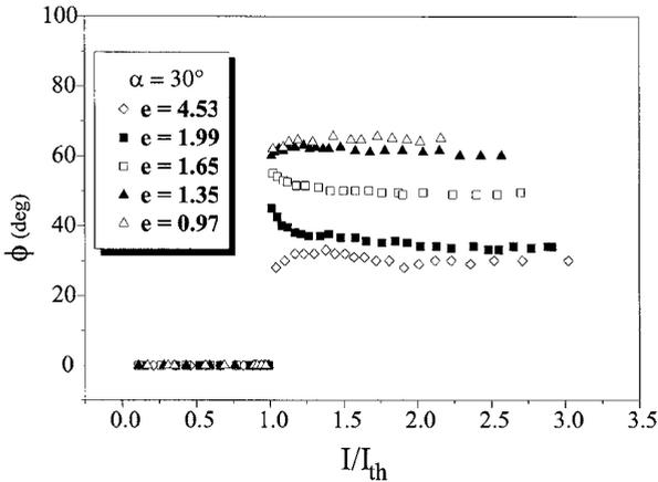
**Figure 6.** Steady-state value of the director average azimuthal angle  $\phi$  as a function of the reduced laser intensity  $I/I_{th}$  for different values of  $e$  of the unpolarized beam spot at the sample. The spot ellipse major axis was oriented at  $\alpha = 30^\circ$ . Below threshold ( $I/I_{th} < 1$ ), the angle  $\phi$  has no physical meaning.
