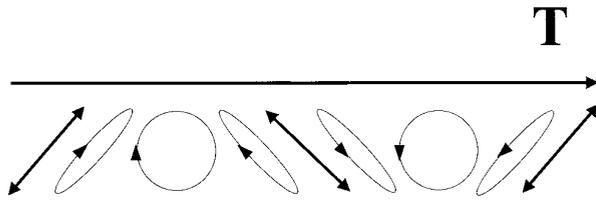
**Figure 5.** Polarization state sequence in our artificially depolarized light.
