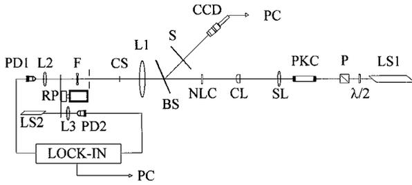
**Figure 4.** Our experimental apparatus. LS1, LS2, laser sources; P, polarizer; PKC, Pockels cell; SL, spherical lens; CL, cylindrical lens; NLC, liquid crystal sample; S, screen; BS, beam splitter; CS, circular spot; F, neutral filter; L1, L2, L3, lenses; PD1, PD2, photodiodes; RP, rotating polarizer; PC, personal computer.
