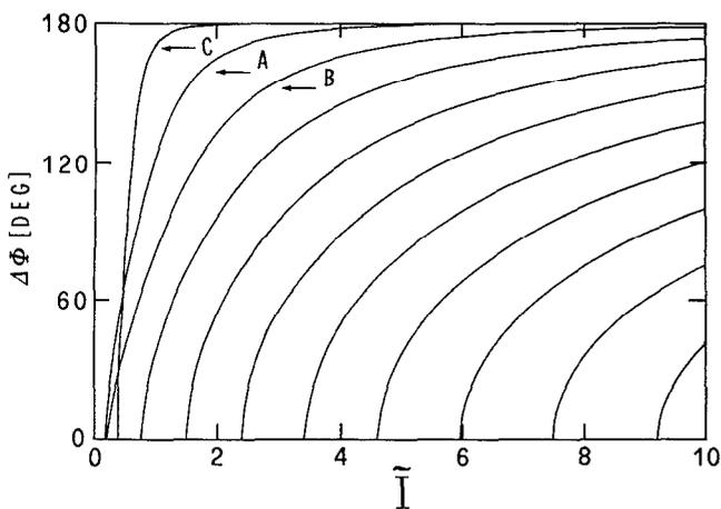
FIG. 2. Twist angle  $\Delta\phi$  vs the normalized light intensity  $\bar{I}$  for an optical sample thickness  $\bar{L} = 2.5\pi$ . Curves A, B, and C correspond to their analogous in Fig. 1.
