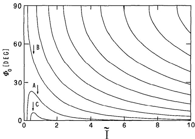
FIG. 1. Rotation angle  $\phi_0$  vs the normalized light intensity  $\bar{I}$  for an optical sample thickness  $\bar{L} = 2.5\pi$ . A, B, and C are the curves originating from the lowest thresholds, respectively.
