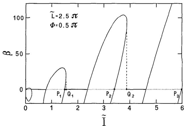
FIG. 3. Plot of the eigenvalues  $\beta_n$  vs the normalized light intensity  $\bar{I}$  for the reference steady state  $\phi = \frac{1}{2}\pi$  and optical sample length  $\bar{L} = 2.5\pi$ . The instability regions of the reference state are dotted. The  $P_i$ 's are branching points not implying the stability change of the solution, which occurs indeed at points  $Q_i$ .
