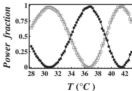
FIG. 2. STOC power fraction  $P_{R,2}/P_0$  (black squares) and no STOC power fraction  $P_{L,0}/P_0$  (empty squares) as functions of the QP temperature. The curve is the best fit obtained as explained in the text.
