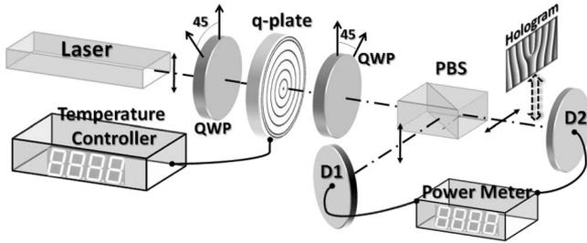
FIG. 1. Setup to measure the STOC efficiency and the state purity. Legend: QWP-quarter wave plate, PBS-polarizing beam-splitter. The fork hologram was inserted on the converted beam arm for verifying the degree of purity of the OAM  $m=2$  mode generated on the output.
