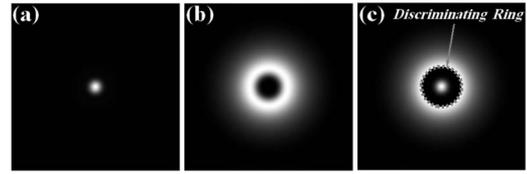
FIG. 3. Calculated far-field patterns of OAM modes  $m=0$  and  $m=4$  generated by the QP for input OAM  $m = \pm 2$  [the input beam was assumed to HyGG<sub>-2,±2</sub>( $r, \phi, 0, 1$ ) (Ref. 18) mode]. The dashed circle shows the discriminating area used in the balanced mode sorter.
