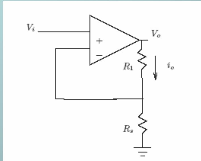
$$V_o = (R_1 + R_s)i_o = \frac{R_s}{(R_1 + R_s)} V_i$$
