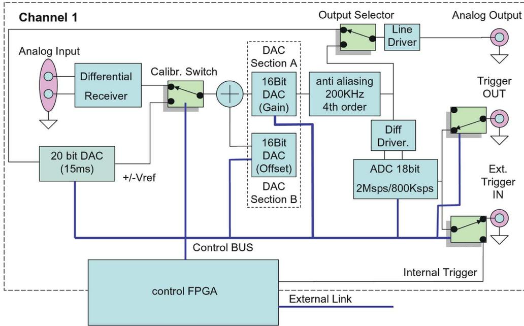
Fig. 1. Block scheme of the acquisition and control daughterboard. In the picture only one channel is shown, being everything but the FPGA duplicated for the other channel. The switches connected to the control bus are managed by FPGA registers, the output selector is set via a jumper. The ADC trigger can be either internally or external generated and, in both cases, can be routed to an output connector.
