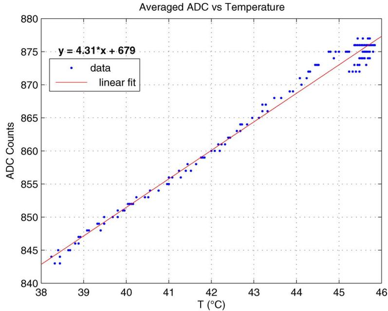
Fig. 5. Value read by 18 bit ADC on a  $50\ \Omega$  load versus the temperature read by 14 bit ADC reading the on-board temperature probe. The board has been placed into an electric oven and the measurements have been taken every second while the oven temperature was rising.
