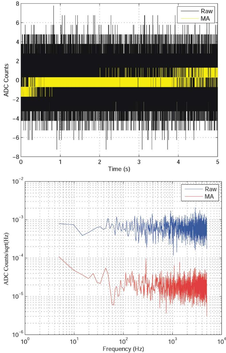
Fig. 4. Internal noise acquired at 10 kHz raw and filtered with the moving average and power spectral density of the two data series. The moving average operation lowers the noise level of a factor  $\sim 10^2$  at this frequency (1 count =  $20 \text{ V}/2^{18}$ ).
