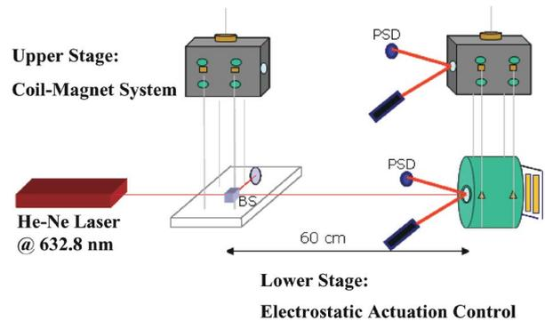
Fig. 6. Suspended Michelson interferometer.
