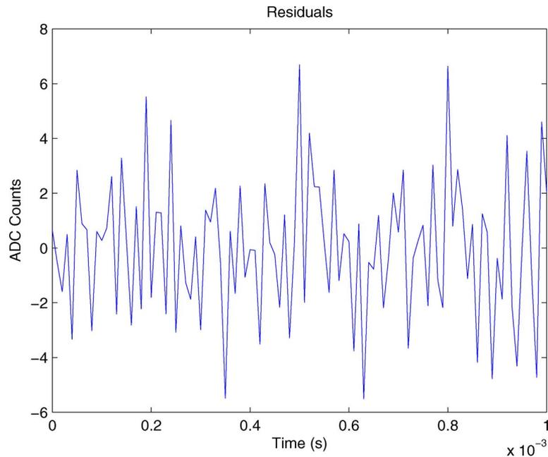
Fig. 2. Difference between the ADC read value and the input sine wave for 120 mV amplitude. The input sine wave estimation is the result of a fit. The maximum value of the residual is a result of the sampling step and the input signal slope.
