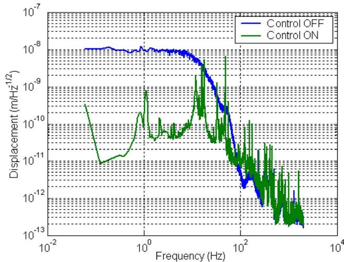
Fig. 8. Preliminary results of the suspension lower stage control with electrostatic actuators. The power spectral density of mirrors' relative displacement are shown both with and without the lower stage control. The peaks in the controlled power spectrum are due to residual mechanical rotational-translational modes coupling and violin modes.
