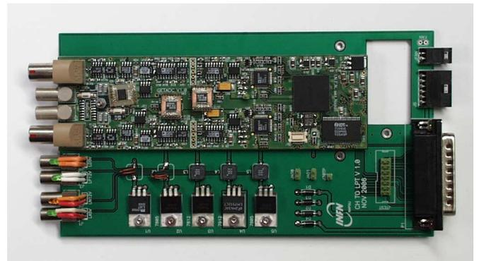
Fig. 3. Prototype of the module with the power distribution board. The hole in the power distribution base is to host the fan.
