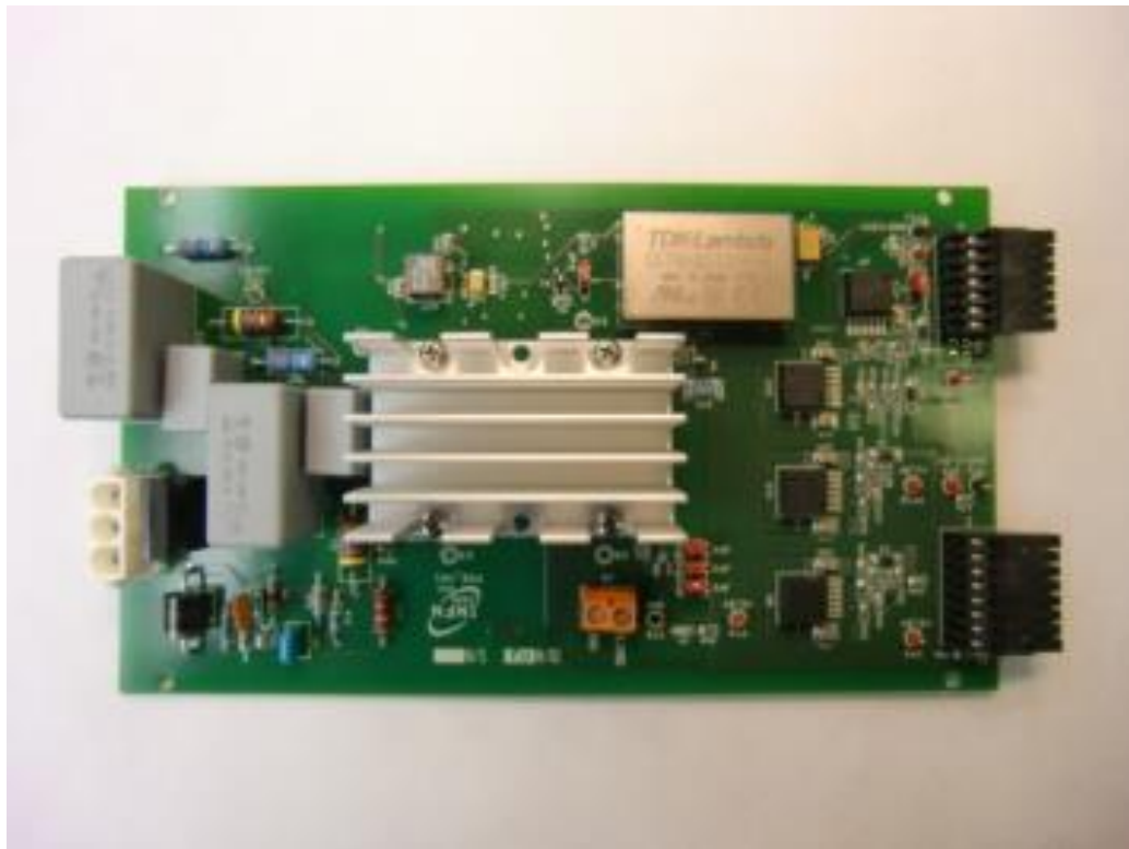
Fig. 4.9: First release of the power system board
