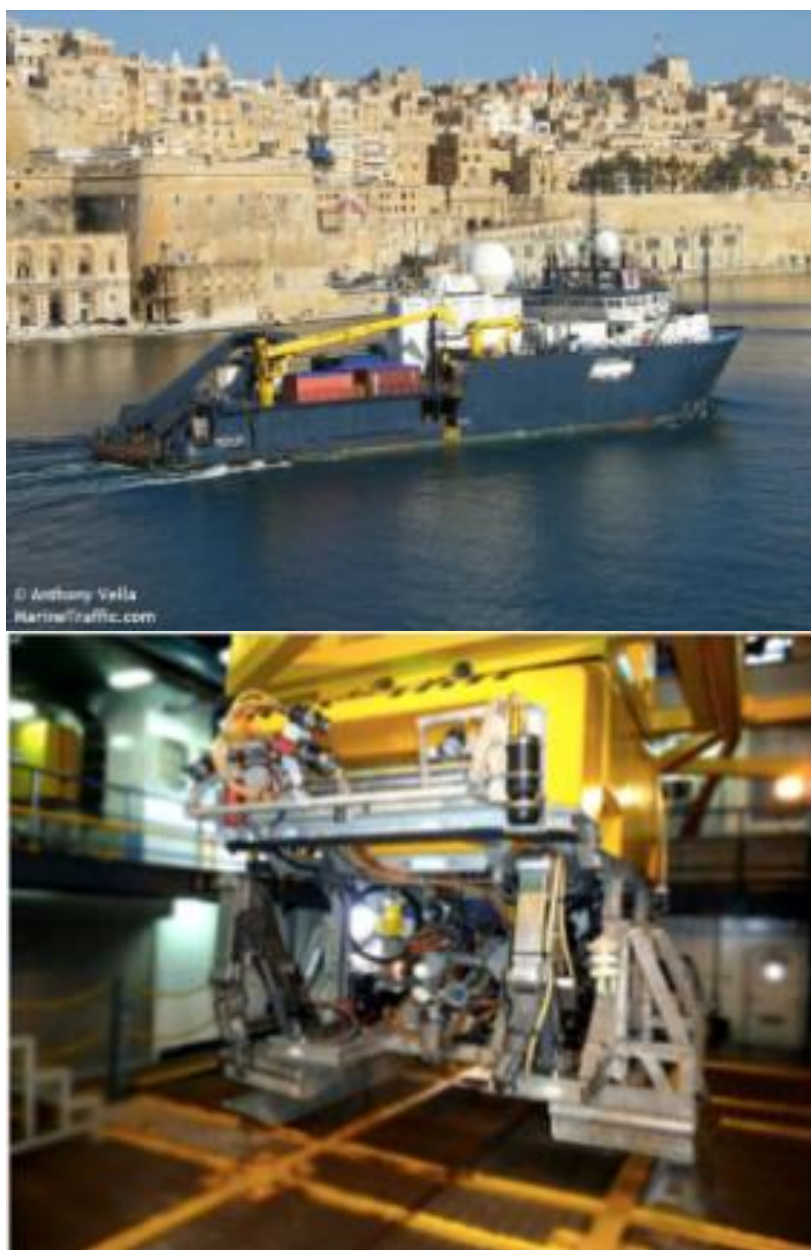
Fig.2.4: the the Multi Service Vessel named Nautical Tide from FUGRO in front of Malta (upper part); the heavy work class ROV rated up to 5000 mwd (lower part).
