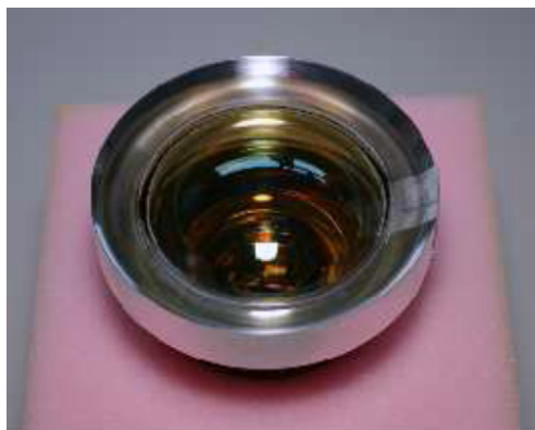
Fig. 3. Expansion cone mounted on a PMT.
