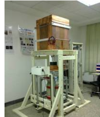
Low background gamma spectrometer in IHEP
