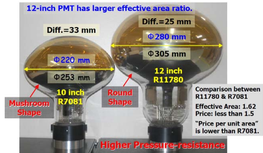
12" PMT with SBA photocathode--Hamamatzu
