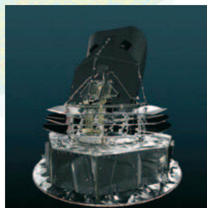
The Planck satellite: an intricate maze of pipes, wires and waveguides connects the warm and cold parts of the satellite.
