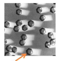
**AgBr crystal**, size 0.2-0.3 micron Is the elementary detection element
