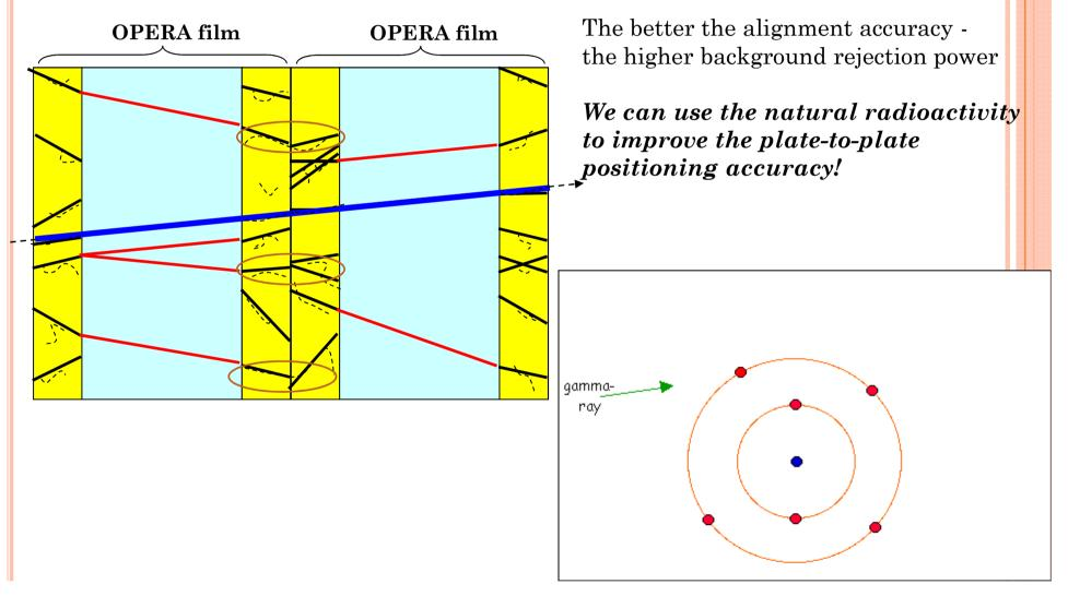
Compton alignment map for one Changeable Sheets doublet Area of 70 cm<sup>2</sup> fully scanned on both CS 2 millions mt/pattern are divided in 414 zones of 4x4 mm<sup>2</sup>, 258750 elementary alignments done to produce this map *Accuracy gain: from 15 microns to 1-5 microns : overall BG reduction is of the factor of 25*
