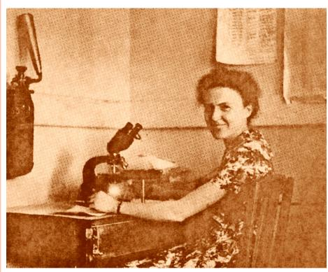
Before 1974 – the only way to find the charged particle tracks and decays in the nuclear emulsions was the eye inspection using manual microscopes
