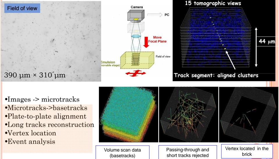
The full offline processing chain for the emulsion data was developed in Napoli (FEDRA system)
